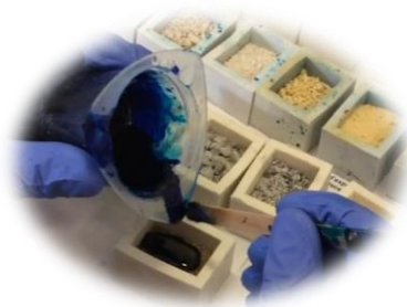
Resin impregnation for highly brittle and friable rocks
